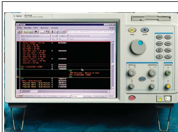
16700 Logic Analyzer With PCI Express Packet Analysis and Other Bus Probes
